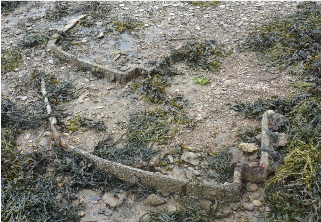
Figure 15: Iron knees that have become detached from the vessel, they show the curve of the hull up to deck level
