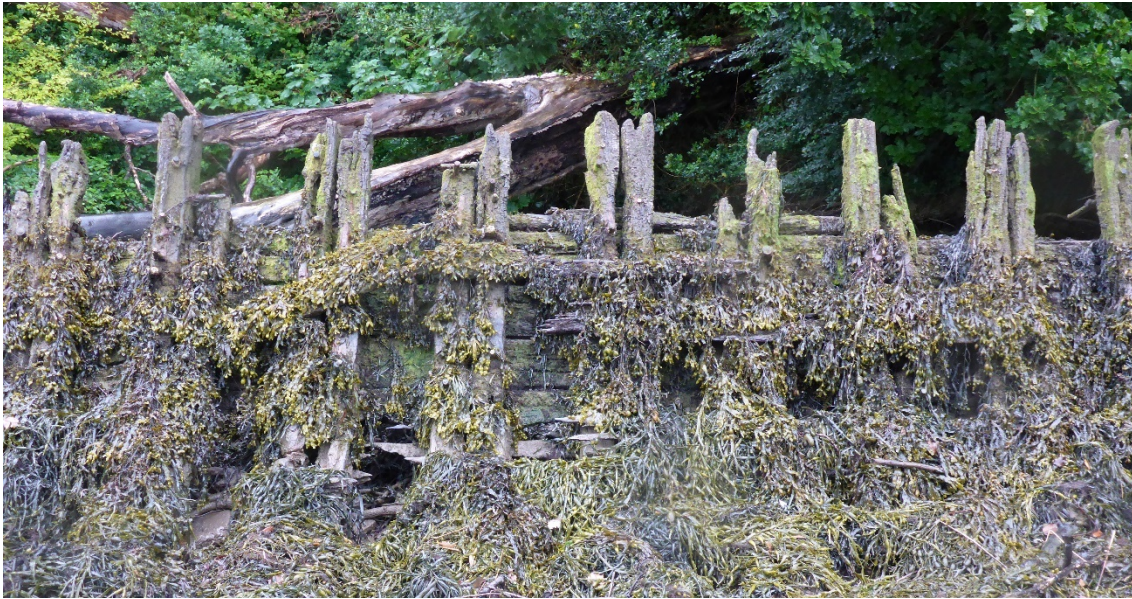
Figure 23: Hull side with paired frames, fastenings can be seen where ceiling planking has gone, lateral fixings between frames also visible
