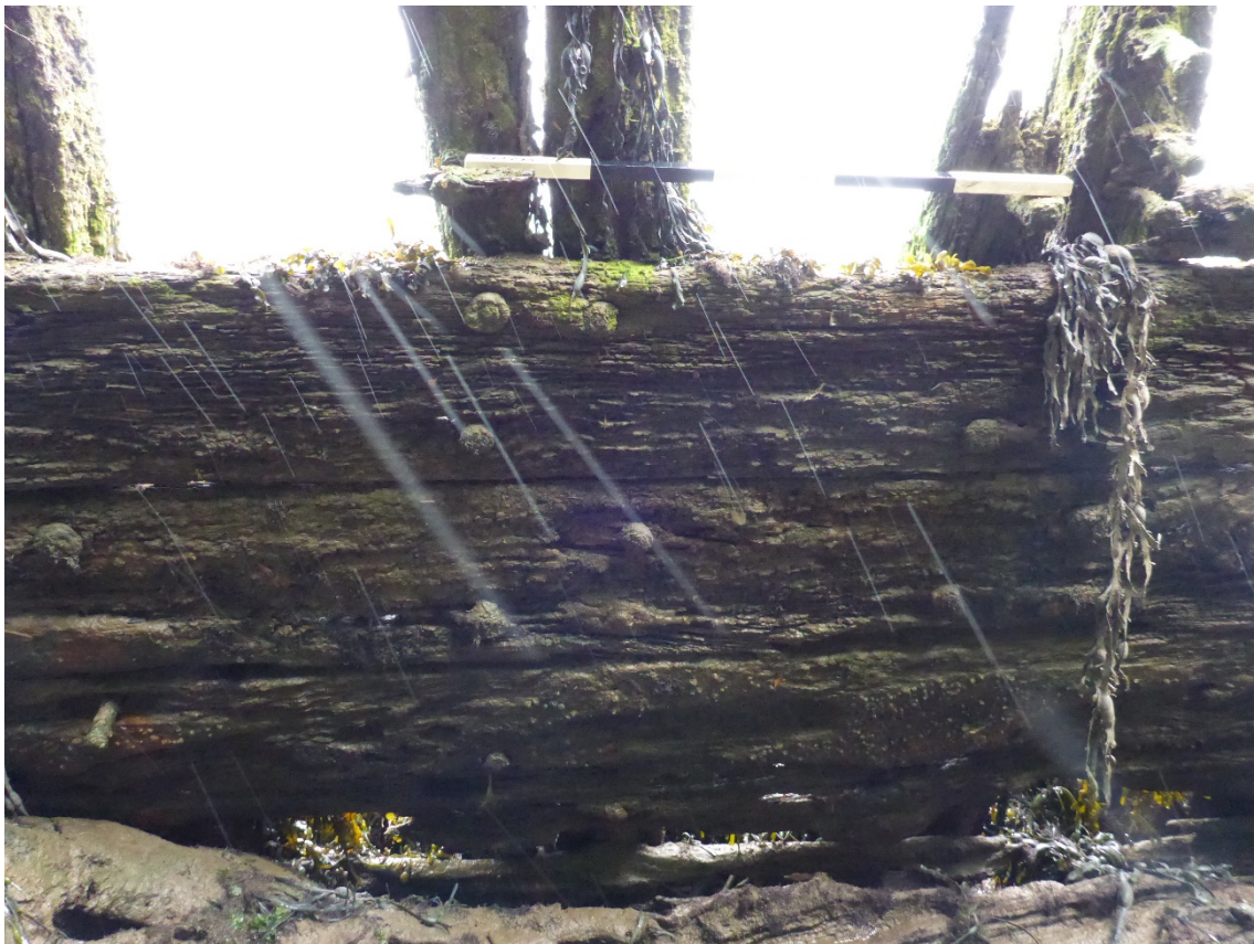
Figure 24: Outer hull planking showing the pattern of fastenings through to the frames
