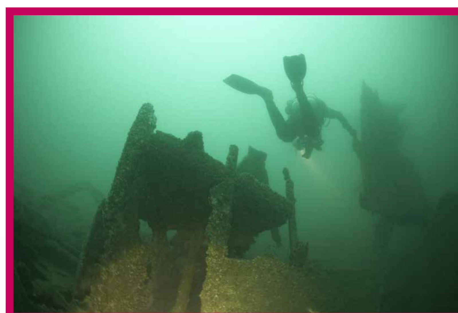
Right: the boilers of the SS Londonier . The Londonier had a triple expansion steam engine: steam was fed through three successive cylinders of increasing size and decreasing pressure. They were the most common type of engine seen on steam ships during the 'golden age' of steam. Photo courtesy of Hamish Morrison.
