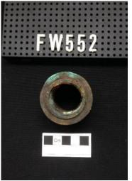
Thought to be from: UC-92 Bearing case Dimensions (mm): L 39, Diameter 52, weight 206g
