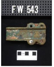
Thought to be from: UC-92 Bracket with multiple fixing holes Dimensions (mm): L 103, W 55, H 21, weight 556g
