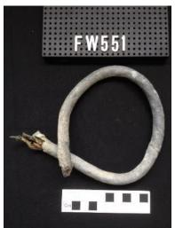
Thought to be from: UC-92 Lead covered wire Dimensions (mm): L 490, Diameter 16, weight 272g
