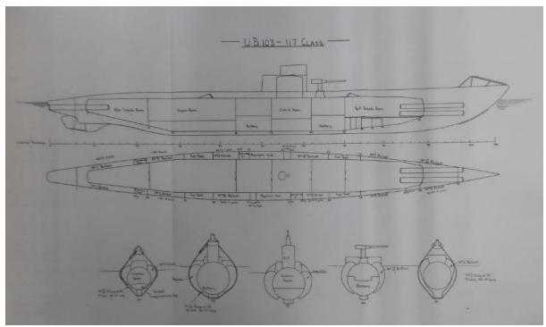
Figure 1: Diagram of a UB III Type submarine (TNA, ADM 189/102)
