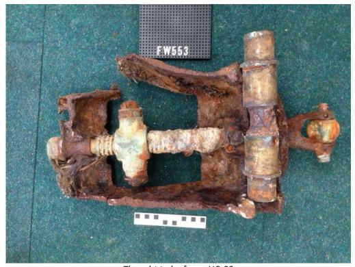
Thought to be from: UC-92 Composite screw mechanism, possibly related to trimming of submarine Dimensions (mm): L 567, W 280, H 215
