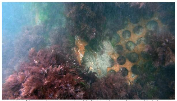
Figure 8: Part of the boiler, the holes once contained the fire tubes, the curve of the edge of the boiler can be seen to the left of the fire holes
