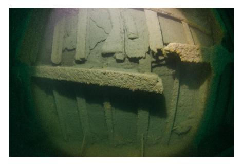
Figure 31: Extant deck near the windlass
