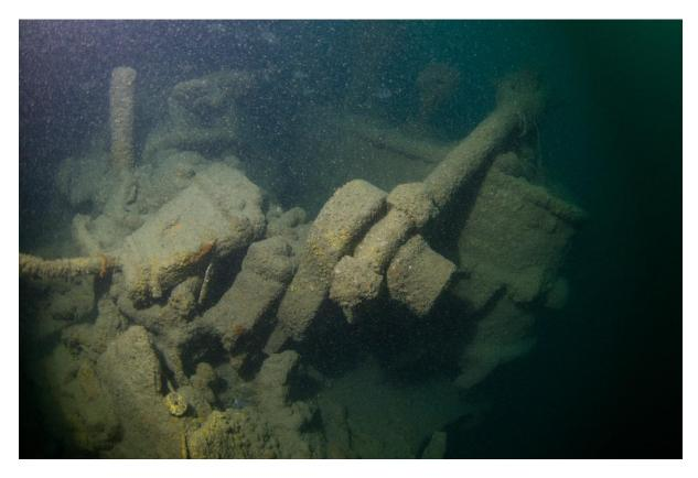
Figure 23: Engine from port side. Centre foreground: crankshaft bearing for the low pressure cylinder. The connecting rod is still attached to the cylinder. The cylinders lie upside down in background.
