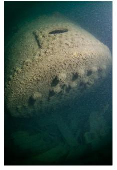
Figure 20: Top of starboard boiler, aft end
