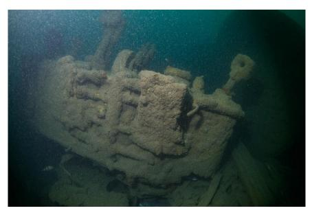
Figure 24: Engine from starboard side, cylinders bent over so the top of the cylinders are now on the seabed. HP cylinder to right/forward. Boiler in background to the right.
