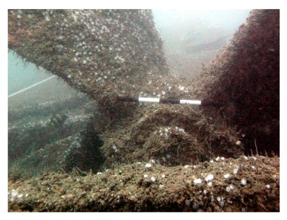
Figure 7: Propeller showing the propeller boss
