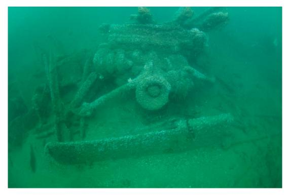
Figure 12: Windless near the bow
