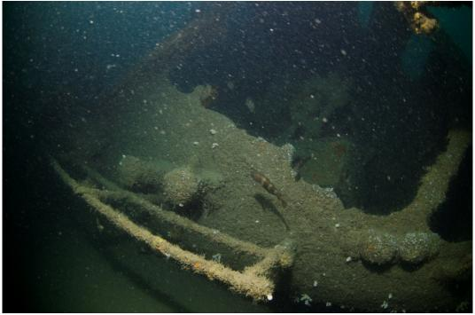
Figure 6: Bollards and starboard rail near the bow
