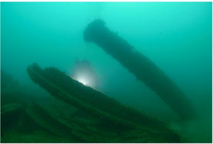
Figure 14: Areas of collapsed hull structure (courtesy of Michael Pitts)
