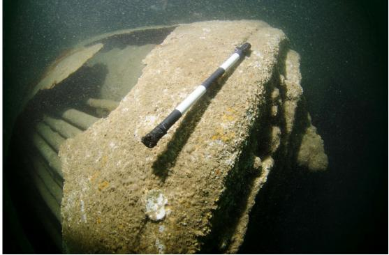
Figure 9: Fire tubes evident through casing
