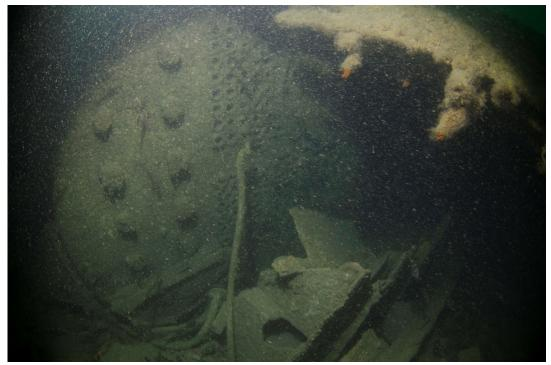
Figure 8: Boiler with hull plating resting on it
