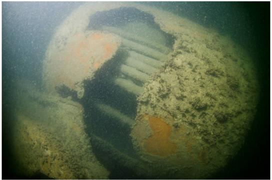
Figure 11: Plan view of horizontal boiler showing damage to the casing and the fire tubes visible inside
