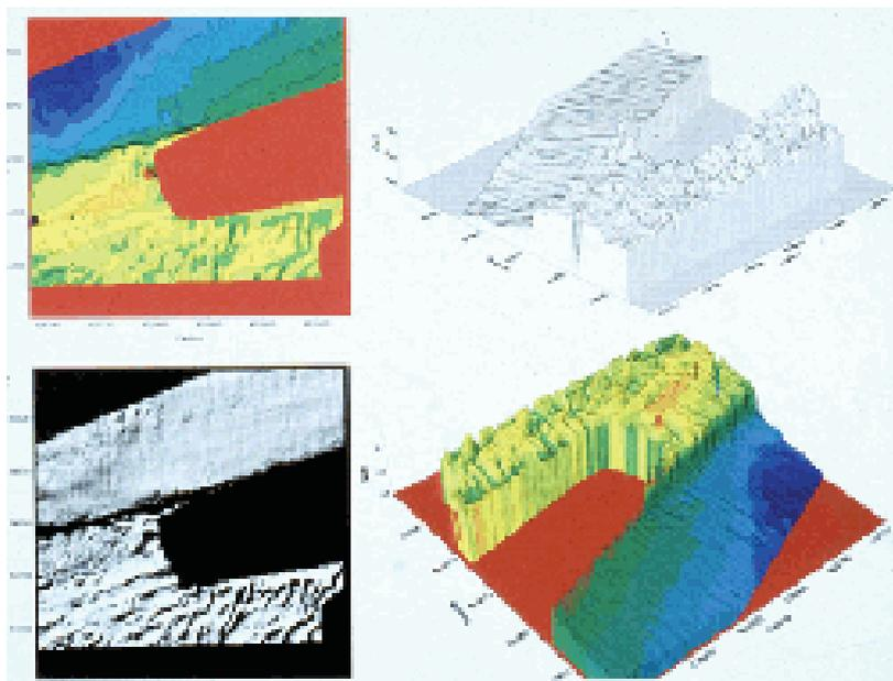
Figure 6 - Images of the Needles from ISIS 100 swath bathymetric survey data
