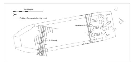
Figure 4.17. Current site extent/remains, overlaid on the outline of an LCT MkV, to illustrate the extent of lost structure.
