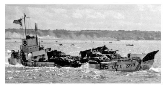
Figure 2.1. LCT(A) 2237 of the US Gunfire Support Group off Omaha Beach on D-Day, the vessel is carrying two Sherman tanks in the firing position with a tank-bulldozer behind them (Source: Robert Hurst, via <a href="www.navsource.org">www.navsource.org</a>).
