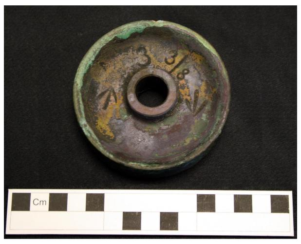
Figure 13. Brass sheave (pulley wheel) stamped with a broad arrow and diameter markings.
