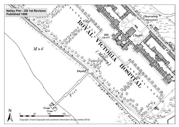
Figure 6. First Revision OS map, published in 1898, showing the disposition of the iron pier on the foreshore in front of the main hospital building (Copyright: Crown Copyright and Landmark Information Group 2015).
