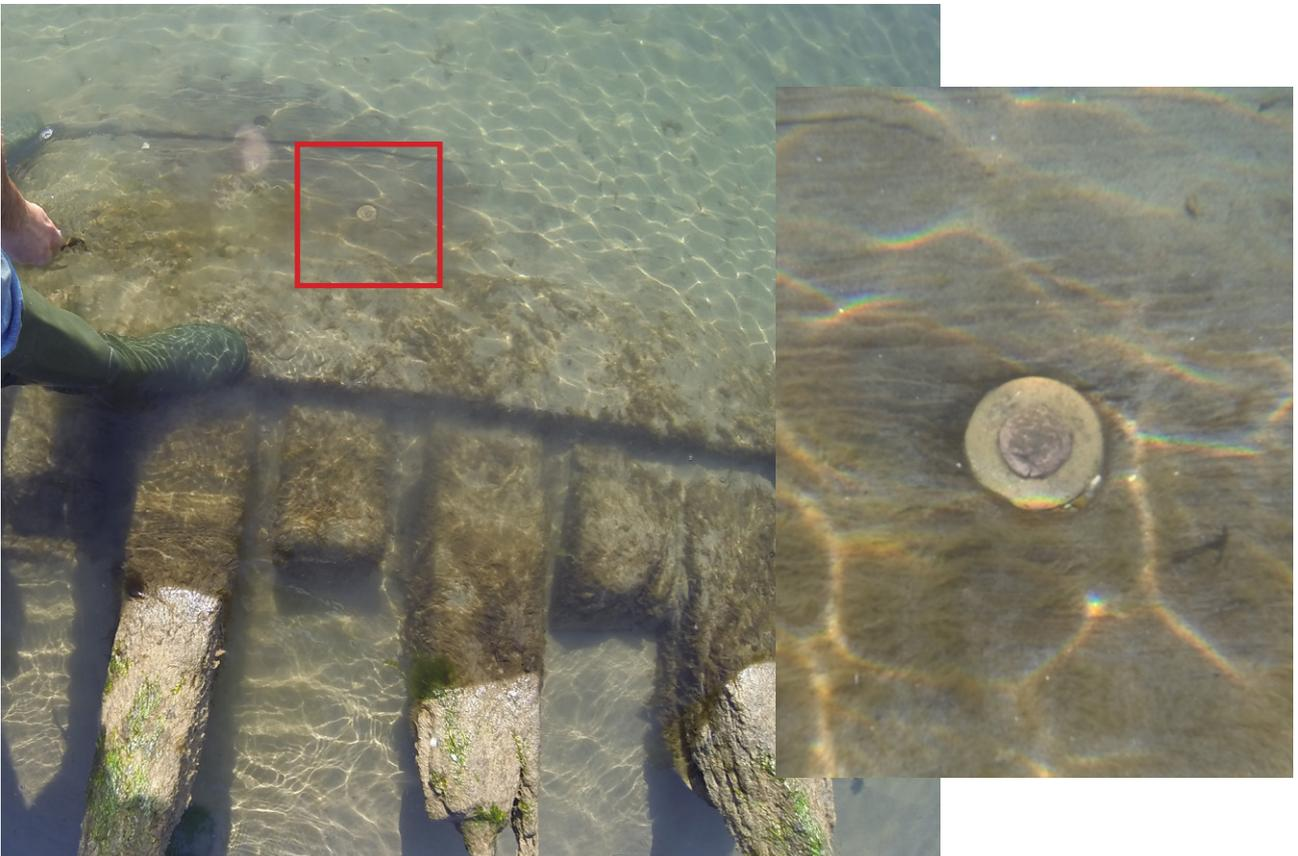
Figure 11. A pair of copper bolts and non-copper washers were used to replace the original wedged treenails that fasten the ceiling planking in place. Inset: detail.
