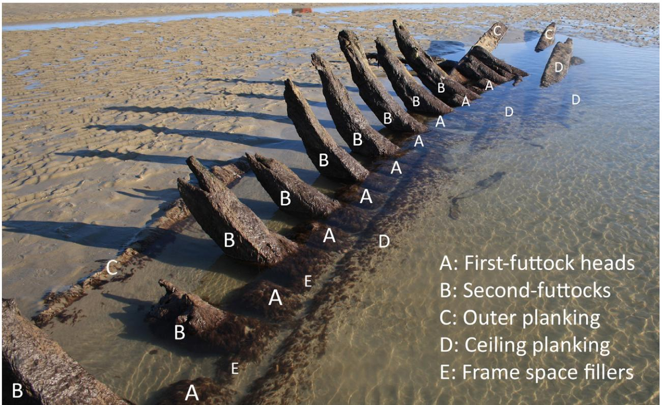
Figure 6. Overview of the wreck, looking south-east towards the bow, annotated with an interpretation of the main structural components observed during site visits.
